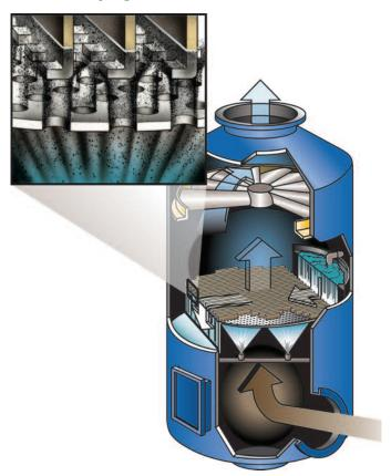
Airflow is drawn into scrubber and passes through plate water, which traps contaminants. These designs are suitable for applications that require collection of both particulate and gaseous contaminants.
